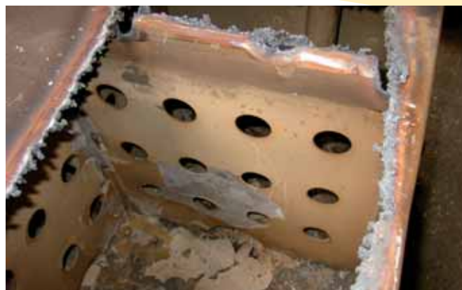
Sediment and debris on walls and bottom of water tank — Source: ISPESL
