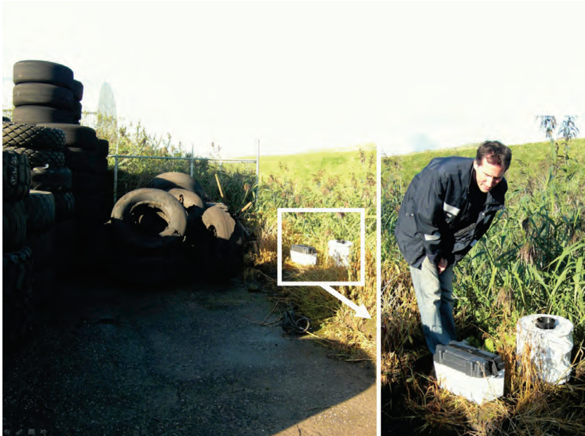
Above: Odour-baited adult trap (BG-Sentinel) at a storage site for used tyres
