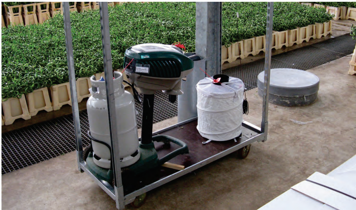
Above: Combined odour- and CO 2 -baited adult traps (Mosquito Magnet) at a greenhouse for Lucky Bamboo
